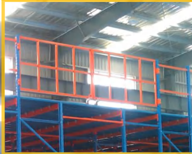
Baluster/ double acting door
